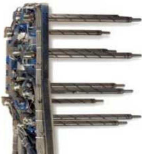
The sheathed thermocouples consist of two dissimilar metal wires welded together and embedded in highly compacted magnesium oxide within a stainless steel housing. The measuring point of the thermocouple can be welded with the sheath thus providing a ground connection. Or it can be supplied ungrounded and insulated from the sheath.
